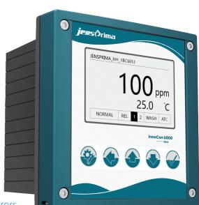
The innoCon 6800I intelligent controller is designed for water treatment and industrial process monitoring. The innoSens ion selective electrode measures ion concentration and temperature in water. PT1000 automatic temperature compensation, more installation method, standard 4-20mA/RS485 and a variety of control function output. Chinese and English menu, user can Self programming.
